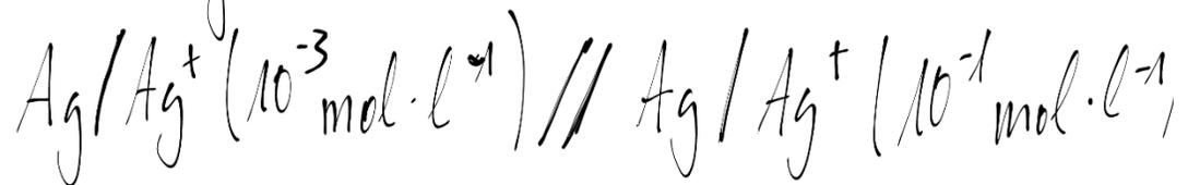
$$c_1: U_H(\text{Ag}/\text{Ag}^+) = U_H^0(\text{Ag}/\text{Ag}^+) + \frac{0,059 \text{ V}}{z} \cdot \lg(c(\text{Ag}^+))$$
